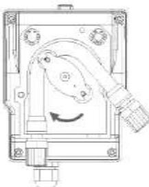
**UK** Insert the left connector into the relative housing and verify that the round part of it will take his position towards the back of the pump. Turn clockwise the roller holder so that the hose will take is natural position in the pump head.
